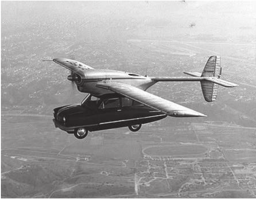
The Convair Model 118 ConvAirCar (also known as the Hall Flying Automobile) was a prototype flying car. The first prototype, piloted by Reuben Snodgrass in 1947 made a low fuel forced landing near San Diego, California destroying the car body and damaging the wing. "The pilot, who escaped with minor injuries, reportedly took off with little or no aviation fuel aboard. Although the fuel gauge he had visually checked during the pre-flight check indicated that the tank was full, it was the automobile's fuel gauge, not the aircraft's gauge." Source: https://wikimili.com/en/Convair_Model_118
